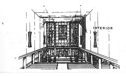
In the 20th century, the acoustics of the interior auditorium are very carefully considered. Note in the PLAN how the two walls of the Nave converge slightly towards the chancel. These angled planes are advantageous acoustically. The suspended ceiling is 32 feet high at the rear, rising to 35 feet at the chancel. The floating ceilings of nave and side aisles do not touch walls or columns, thus suggesting their non-structural character.
